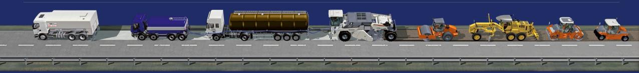
Binder spreader Water tanker truck Bitumen tanker truck Recycler
